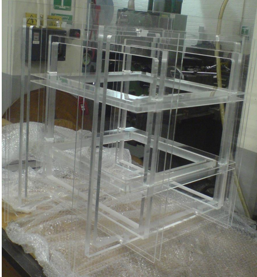
Figure 12.5. Photograph of three-axes Helmholtz coils made with perspex.
