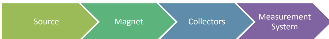
Figure 6.1: Key components of a Mass Spectrometer (Allègre and Sutcliffe, 2008)
