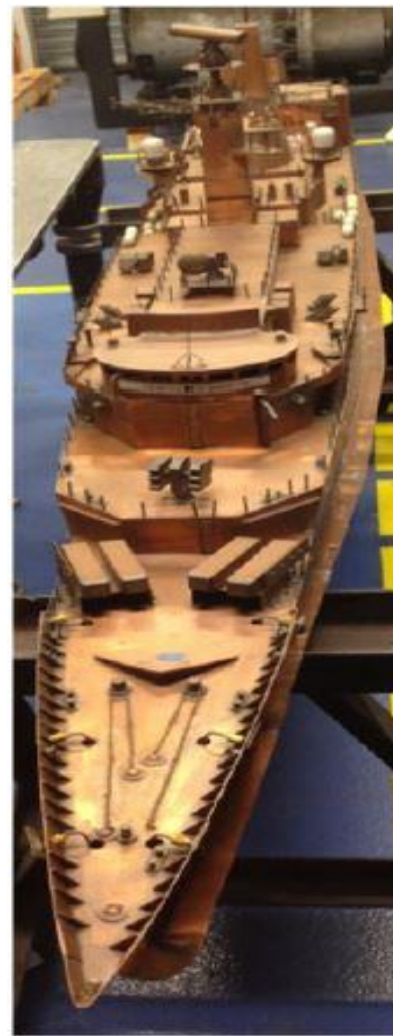
Fig. 7. 1:50 physical copper scale model for the Type 22 Batch II Frigate
