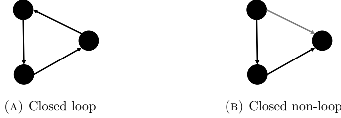
FIGURE F.1: Schematic of closed (left, not allowed) and non-closed (right, allowed) directed pipeline networks between nodes, adapted from Mehleri et al. [96].
