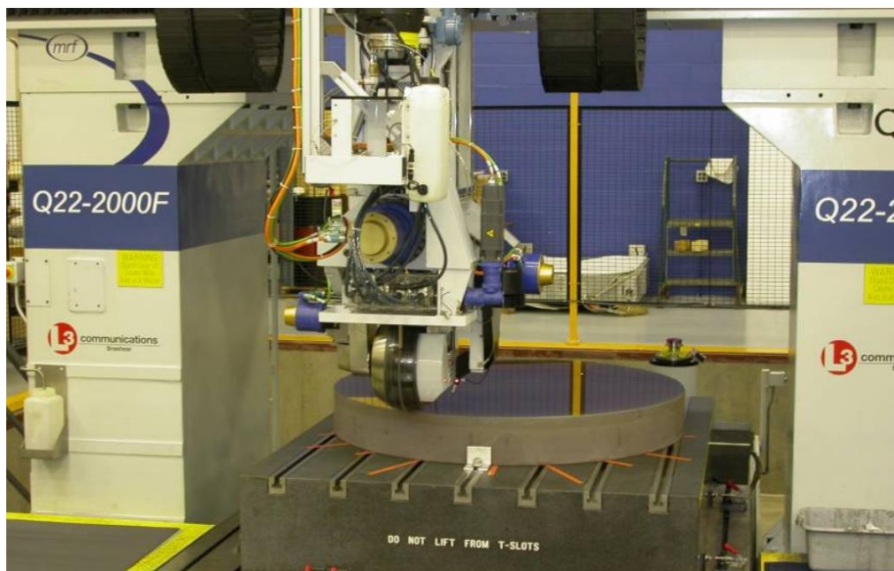
Figure 2-16: QED is used to make a 1.5 m diameter surface [102]
