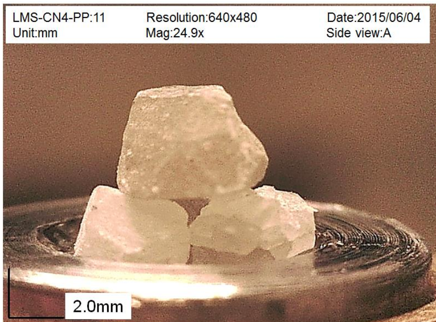
593 Fig. 6 Flat-to-flat contacts between LMS particles.
