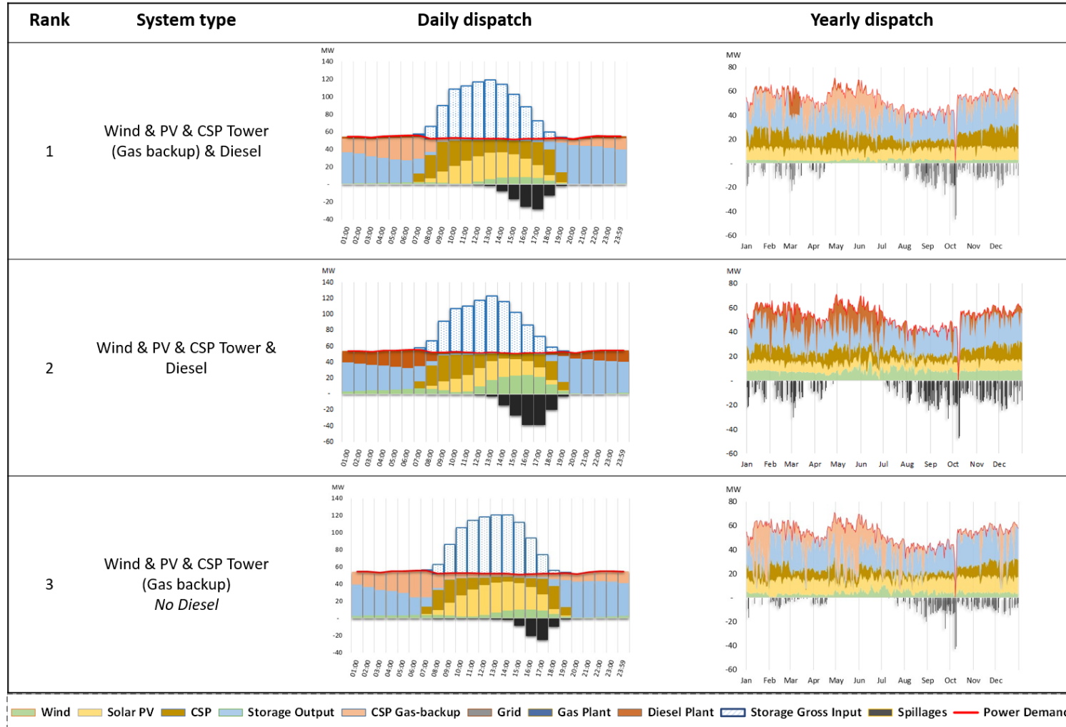
Figure A.3: Power dispatch of optimal technological mixes (1/6): Atacama, Chile (Off-Grid)
