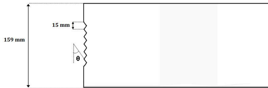
Fig. 4 Schematic design of jagged cut pattern at the leading edge to create uniform spanwise disturbances
