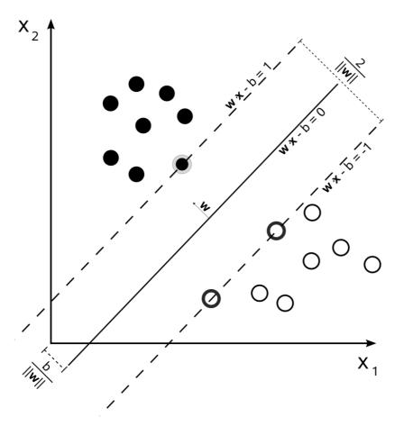
Figure 19: Maximum-margin hyper plane and margins for an SVM trained with samples from two classes. Samples on the margin are called the support vectors.
