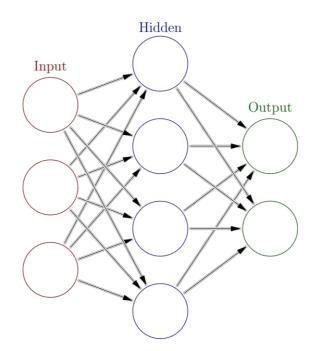
Figure 18: Schematic of a simple artificial neural network showing three inputs feeding into a hidden layer and producing two outputs
