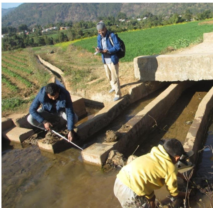
Figure 50. Argauli: locally managed irrigation systems. Debendra Bhattarai (DoA) is measuring the width of canal, while a local boy is managing the water flow, directing water from one field to another using lumps of soil.
