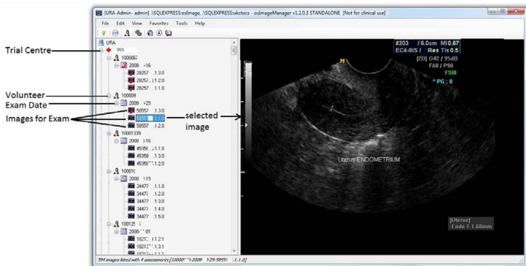
Figure 5-2: osImageManager adapted for Image Review. The images for each exam are contained in the nodes belonging to the volunteer’s exam date. The reviewer double-clicks the exam date node to open the exam assessment dialog box shown in Figure 5-3. Tick marks indicate that the image (or exam) has been reviewed.
