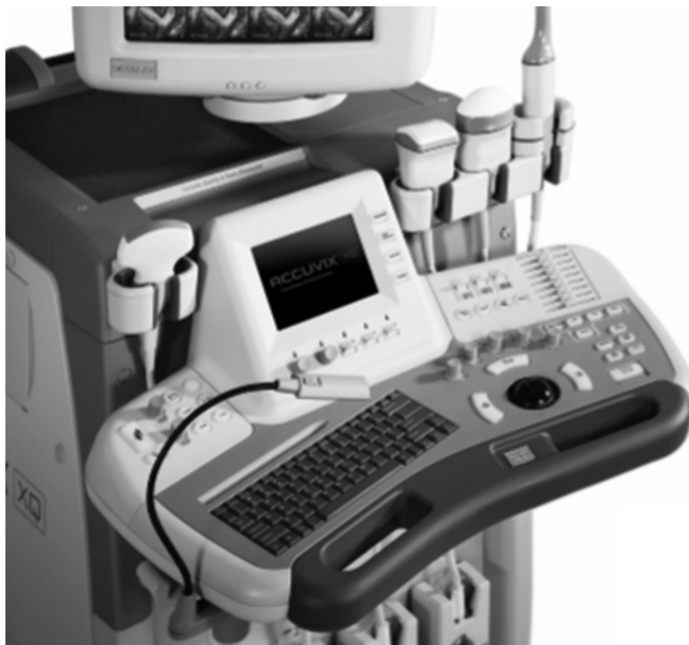
Figure 2-8: Medison Accuvix XQ User Interface is designed to facilitate operation of the machine in a clinical setting. The middle of the picture shows a touch panel containing controls that the machine provides according to the stage of the examination in order to reduce the number of static controls that the sonographer needs to operate. © Samsung Medison Co., LTD. Reproduced with permission.
