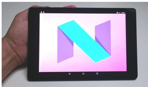
Figure 3. Nexus 9 tablet running Android 7.0 (Nougat) Operating System and a dedicated App for raw GNSS data logging.
