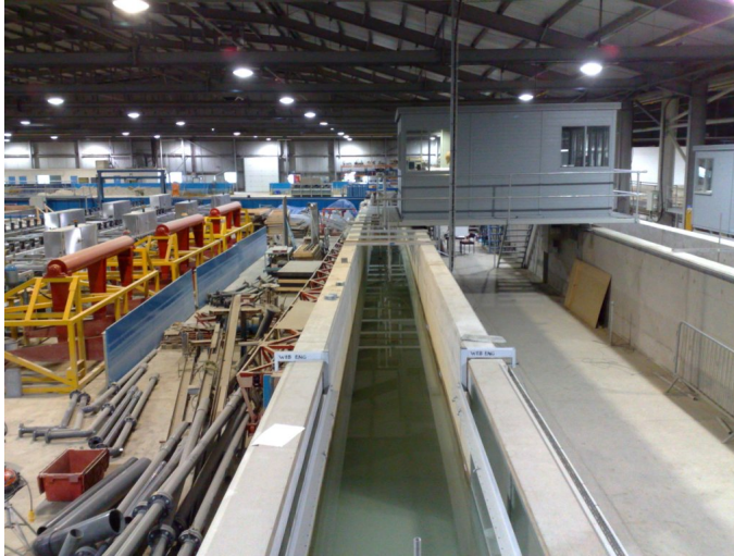
Figure 3.6: 45m wave flume in Froude Modelling Hall at HW Wallingford, photographed from the top of the wave generator.
