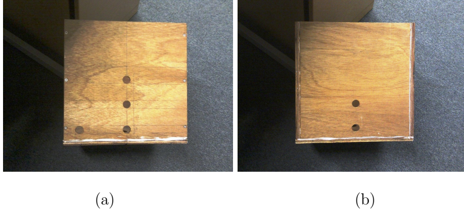
Figure 3.8: Front, (a) and side, (b), of square test structure used to house the six pressure transducers.
