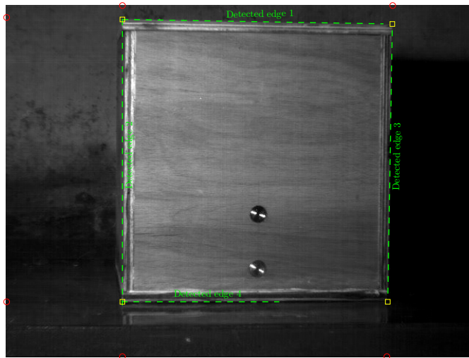
Figure B.3: Edge detection based on peaks of Hough transform visualised in Figure B.2. Corners/coordinate control points (yellow squares) identified by extending the Hough lines to the image limits (red circles). The extended lines are shown in Figure B.4.
