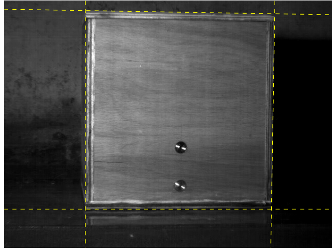
Figure B.4: Average image over-layed with the gridlines defined by edge detection in Figure B.3.
