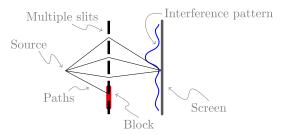
More precisely, this means that the interference pattern created on the screen cannot be written as a particular linear combination of the patterns generated when different subsets of slits are blocked. In the two slit
