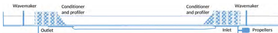
Fig. 1. Schematic side view of the UCL wave-current flume (not to scale) showing two wavemakers at each end of the flume, locations of inlet and outlet of the current discharge, the flow conditioner and the profiler.
