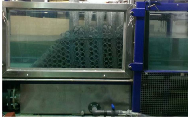
Fig. 2. Photograph of the conditioning and profiling system positioned at the inlet of the flume.
