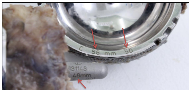
Fig. 6 Photo of the revised Adept hip resurfacing removed from the 53-year-old gentleman. Manufacturer labels in the surgical notes record the components as being a 56-mm cup designed for a 48-mm head and a 48-mm head. Engravings ( red arrows ) and coordinate measuring machine measurements confirm the CSM, as the cup is actually a 56-mm cup designed for a 50-mm head
