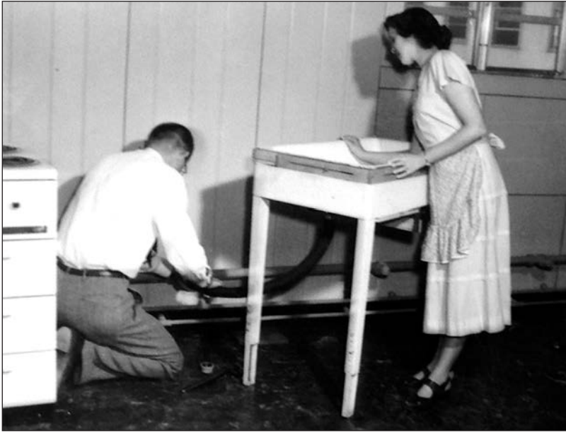
FIG. 7 Publicity photo of “trial run” cabinets in the Housing Research Center Laboratory, 1950. “Mr. L. C. Lamb [Agricultural Engineering] and Mrs. Evelyn Fisher test the arrangement of major kitchen equipment.” Note the height-adjustable sink. (Source: GHB, Box 8.)
