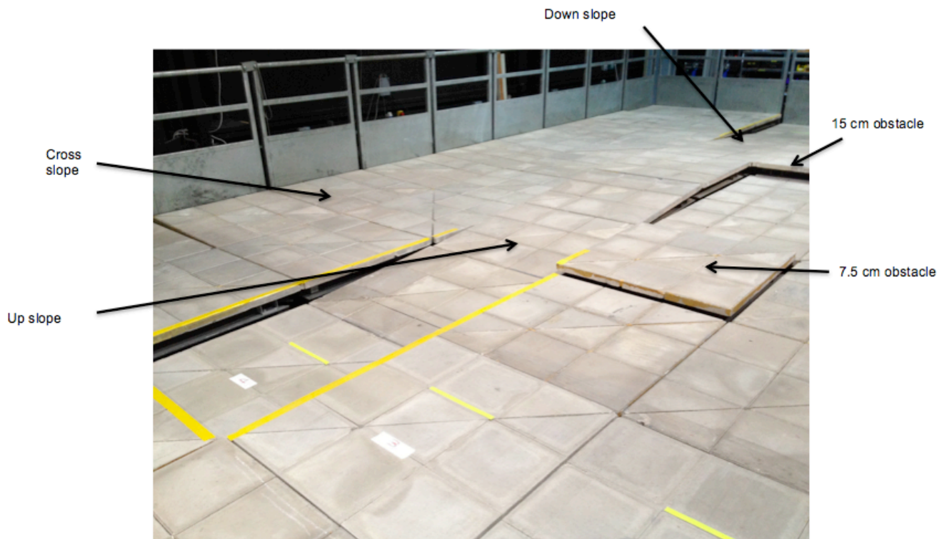
Figure 1. Partial view of the study set-up in PAMELA, illustrating the walkways with obstacles, up and down slopes, and cross slope
