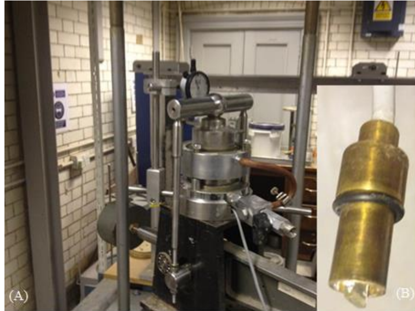
Figure 4-3. a) Oedometer testing system setup for shear wave modulus measurement and b) bender element potted on a brass cartridge.
