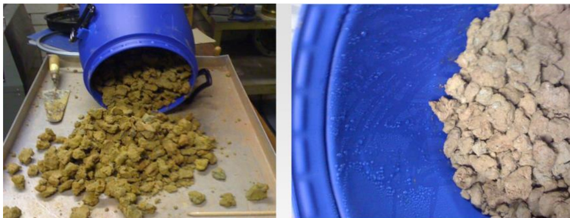
Figure 5-7. Chopped clay peds in storage drum
