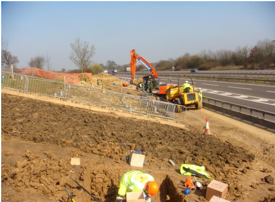
Figure 3-9. UCL Trench for obtaining undisturbed samples
