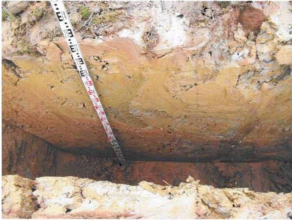
Figure 3-8. Trench 1 mid-slope (view south): Reading Formation (‘lower’ mottled)(Lambeth Group)
