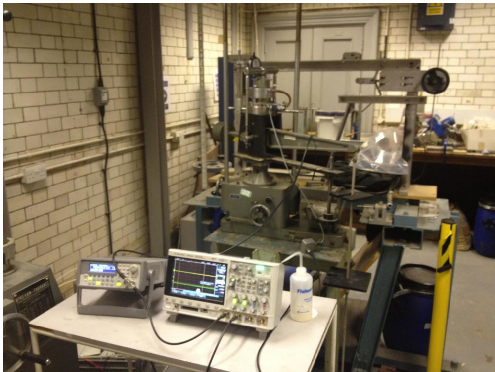
Figure 4-5. Bender element incorporated oedometer testing system setup
