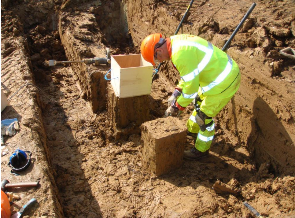
Figure 3-10. UCL UCL Trench- sampling of the the in-situ fibre compacted soil.
