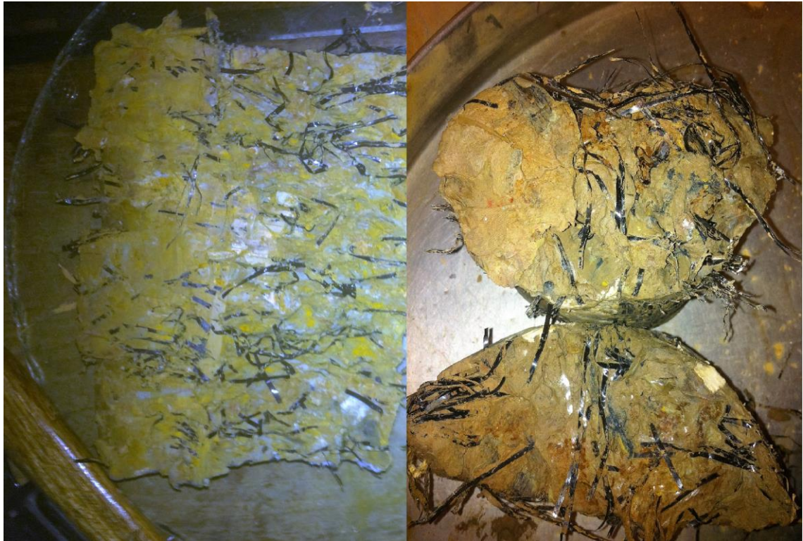
Figure 10-61. Examination of samples after shearing stage
