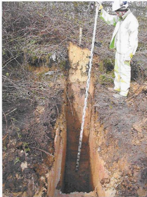
Figure 3-7. Trench 1 at the crest of the slope (view west): Harwich Formation (Thames Group) overlying Reading Formation (Lambeth Group)
