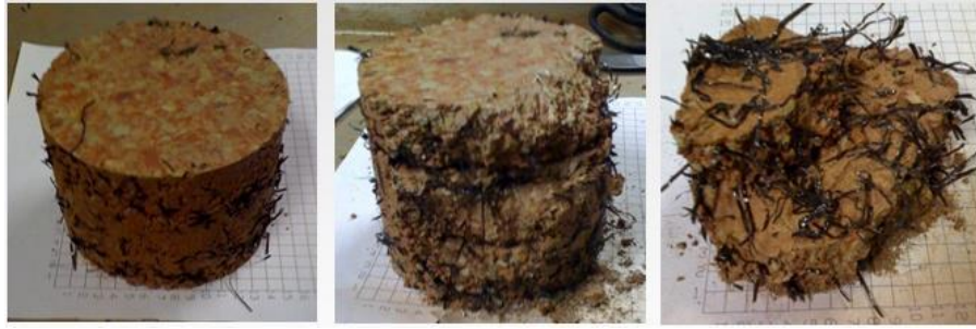
Figure 7-2. Extracting fibres from the sample
