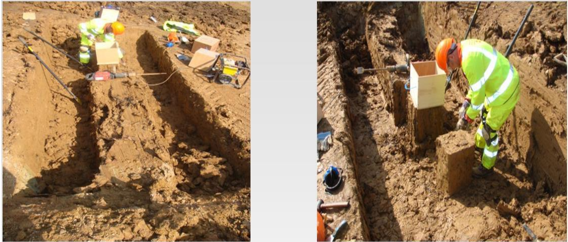
Figure 5-2. Trench for block sampling
