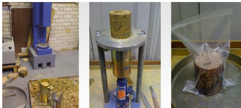
Figure 5-10. Reinforced sample compaction procedure
