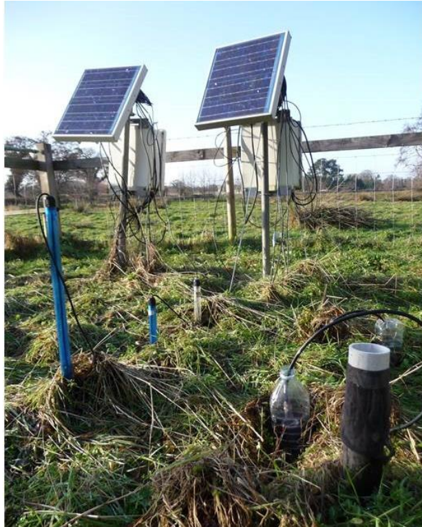
Figure 4.12: Clockwise from top of the photograph, dataloggers, position of the oxygen optodes (protected in plastic containers), and varying depths of the tensiometers.
