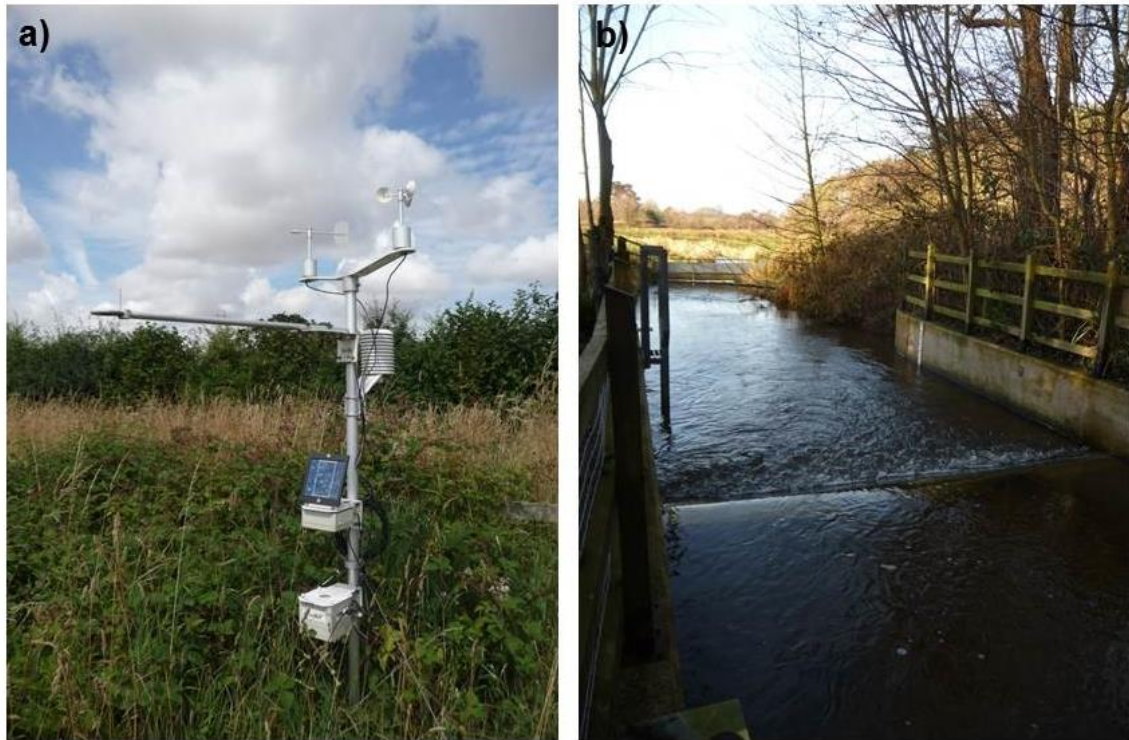
Figure 4.5: Photographs of (a) the automatic MiniMet weather station and (b) the Environment Agency gauging station located at Hunworth (#034052).
