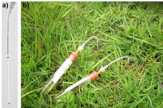
Figure 4.11: Photographs of rhizon soil moisture samplers taken in the laboratory (a), and in the field attached to test-tubes collecting pore-water from the rooting zone.
