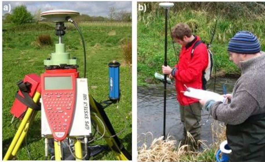
Figure 4.13: Photographs of the differential Global Positioning System base station (a) and the rover in-use at Hunworth Meadow.
