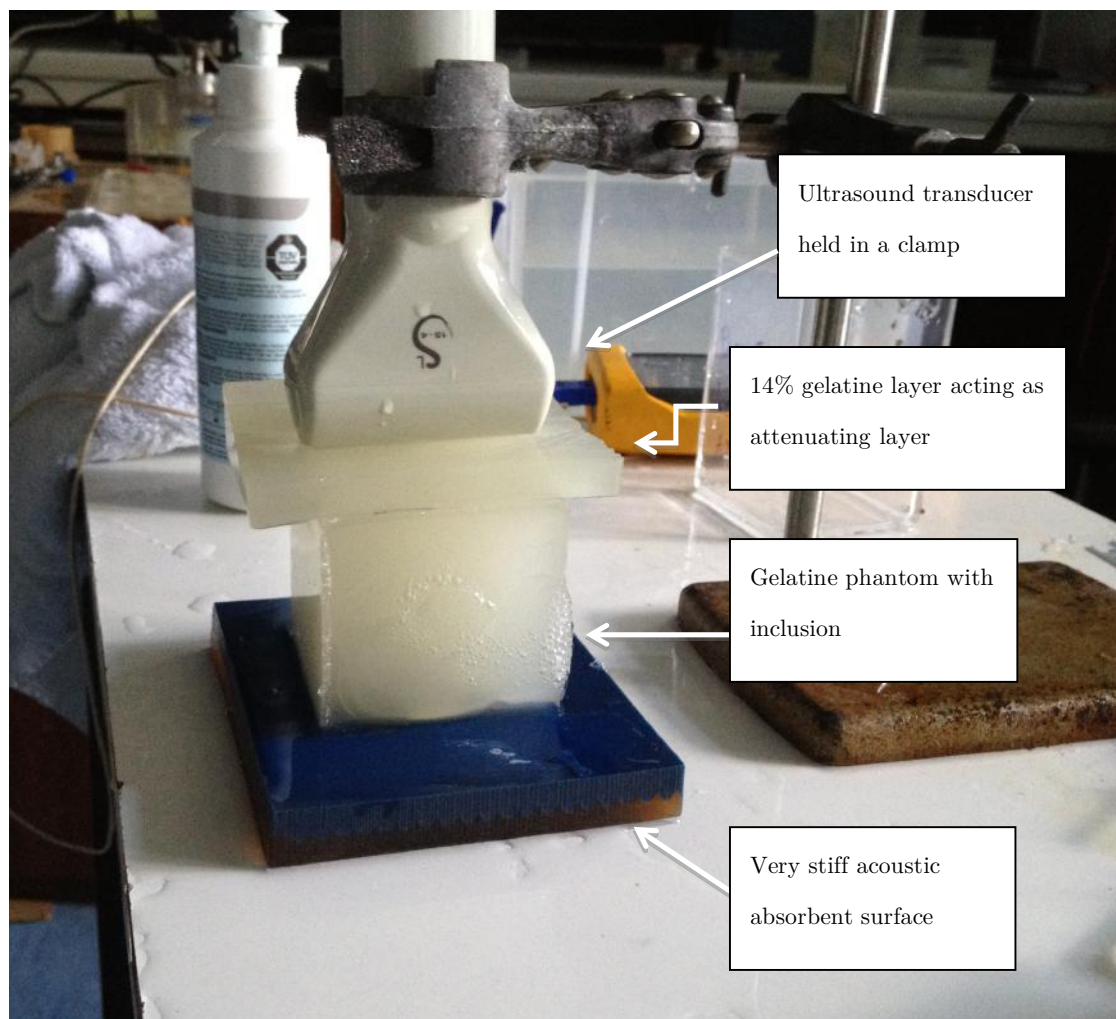
Figure 6.3. The experimental set-up for investigating the effect of attenuating layers on shear wave signal.
