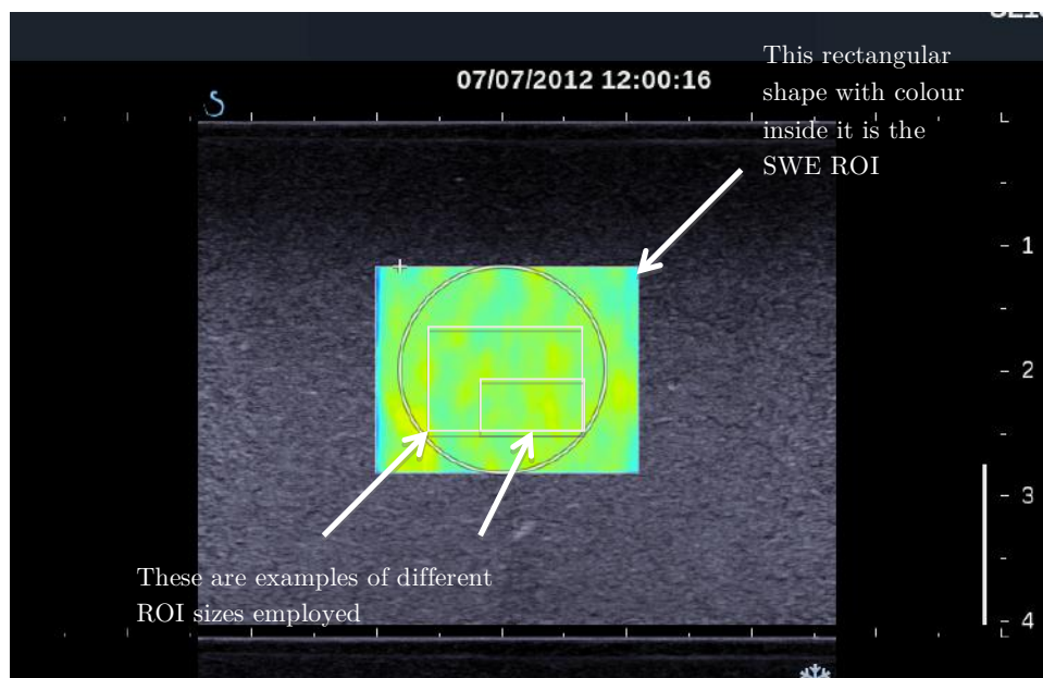
Figure 6.1. This is the top half of the display on the ultrasound scanner where it shows the B-mode image with superimposed colour SWE image within the ROI.
