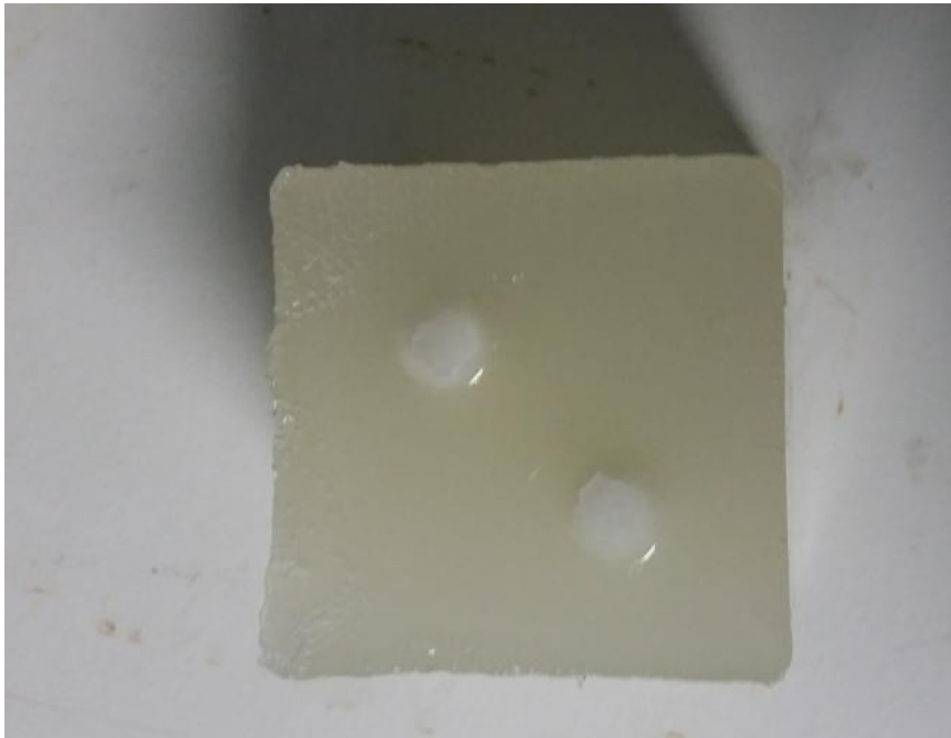
Figure 6.14. Gelatine phantom with 1-cm diameter cylindrical inclusions arranged in diagonal fashion.
