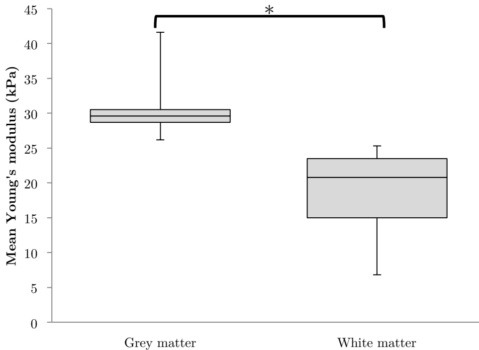
Figure 5.11: The whisker box plot for the mean Young's moduli of normal cortical grey matter and subcortical white matter. The upper and lower bounds of the box were the third and first quartiles, respectively, while the line within the box was the median. The upper and lower whiskers were maximum and minimum, respectively. *Wilcoxon's signed ranks test showed the difference in the mean Young's moduli between the two regions of the normal brain were statistically significant ( p = 0.008).
