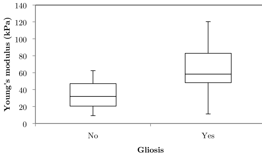
Figure 7.21: Box and whiskers plot of Young's modulus for epileptogenic lesions according to the presence of gliosis (n=21). The upper and lower bounds of the box were the third and first quartiles, respectively while the line within the box was the median. The upper and lower whiskers were maximum and minimum values, respectively. There was no statistically significant difference ( p = 0.185 , Mann Whitney U test).
