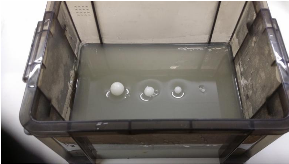
Figure 6.12. Three-dimensional (3D) phantom with small spheres measuring 12 mm, 8.5 mm, 6 mm and 2.5 mm in diameter, from the left, placed on a partially solidified background gelatine. More gelatine will be poured over it to make the phantom.
