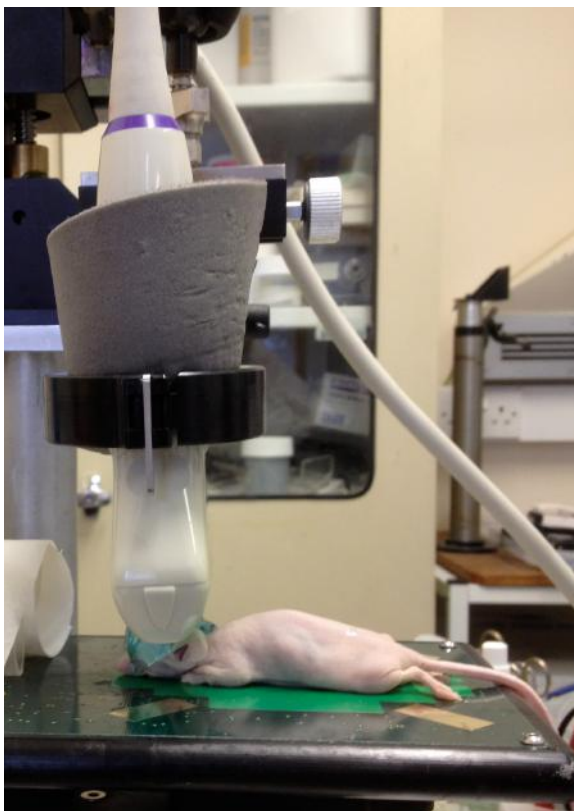
Figure 4.16. A photograph of the setup for SWE acquisition in the brain of a dead mouse.
