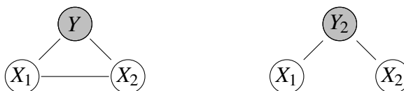
Figure 2.1: Latent variable model (left) and the tractable sub-graph (right) corresponding to a variational approximation. Observed variables are shaded grey.
