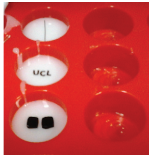
Figure 9. Phantoms are shown before the second layer of PVCP was poured.
