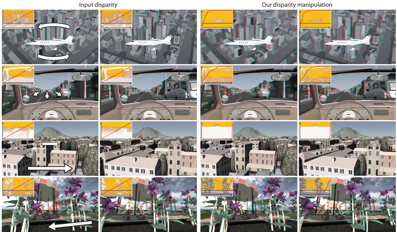
Figure 7: Results of our parallax-aware disparity manipulation applied to four video sequences used in our user study (Sec. 6). The mapping curves along with the output disparity maps are shown in the insets. The blue color marks crossed disparity, yellow uncrossed disparity and white zero disparity. The arrows show the local motion direction.
