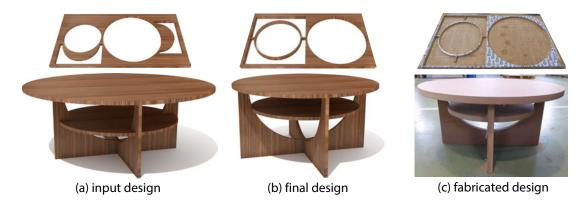
**Figure 5.1:** Waste-minimising furniture design. We introduce waste-minimising furniture design to dynamically analyse an input design (a) based on its 2D material usage (see inset) and design specifications to assist the user through (b) multiple design suggestions to reduce material wastage (see inset). The final user design can directly be exported for laser cutting and be assembled (c). In this case, wastage was reduced from 22% to 11%.
