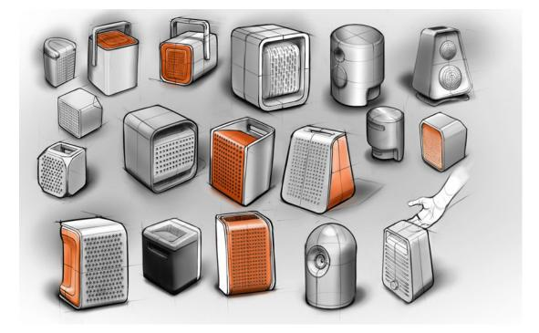
**Figure 2.3:** Concept sketches. Concept sketches are a powerful tool that allows designers to explore the design space effectively. Many sketches with various specifications of the design are produced and compared for the effective exploration of the design space (image by Derick Schweppe).
