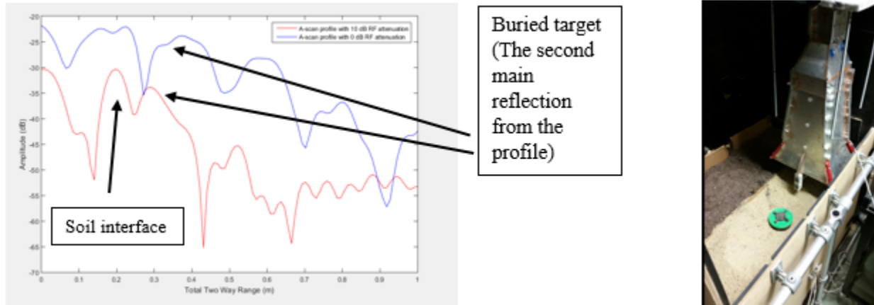
Figure 7-4: Effect of RF attenuation on the A-scan profile applied to the VNA front end
