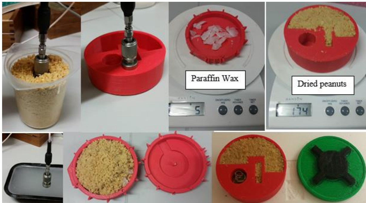
Figure 7-10: Dielectric properties testing and filling of 3D printed models of landmines with dried peanuts and paraffin wax
