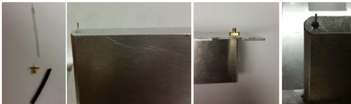
Figure 6-4: Feeding mechanism of the double ridges
