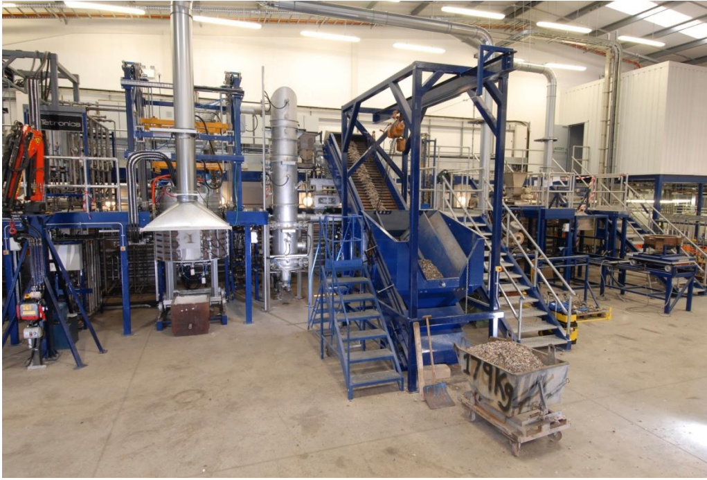
Figure 2.7.2. Pilot plant of the Gasplasma process developed in Swindon for electricity production.
