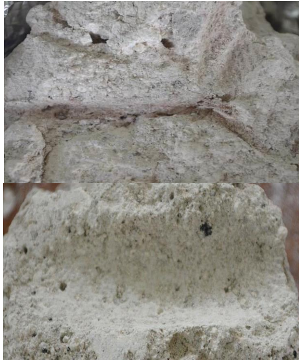
Figure 261 Photograph of wood and stick impressions (photo by Pieta Greaves, courtesy of Tom Guderjan)
