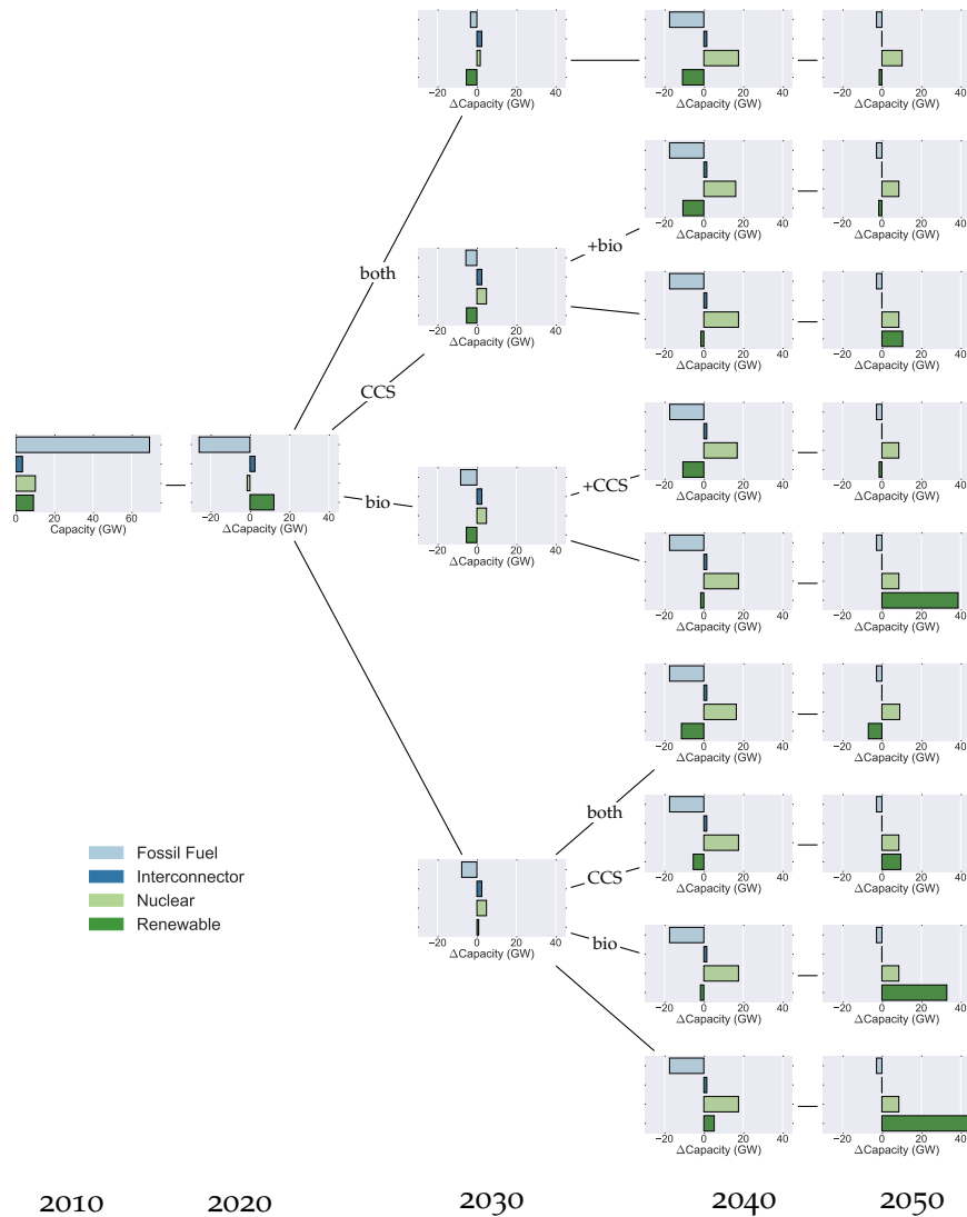
Figure 42: Annual change in capacity over time as a consequence of build rate of CCS and biomass availability
