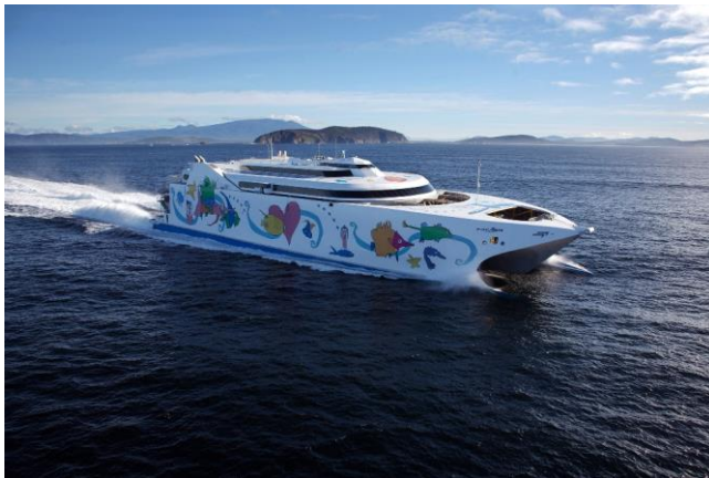
Fig. 1: Hull 064 - Natchan Rera. A 112m INCAT high speed wave piercing catamaran (image courtesy of INCAT Tasmania Pty Ltd).
