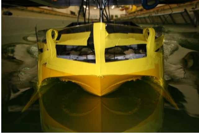
Fig. 5: Formation of jet flows during the water entry of the centre bow on a 2.5m scale model of an INCAT wave piercing catamaran in 90mm waves at a forward speed of 1.53 m/s (Lavroff, J., 2009b).
