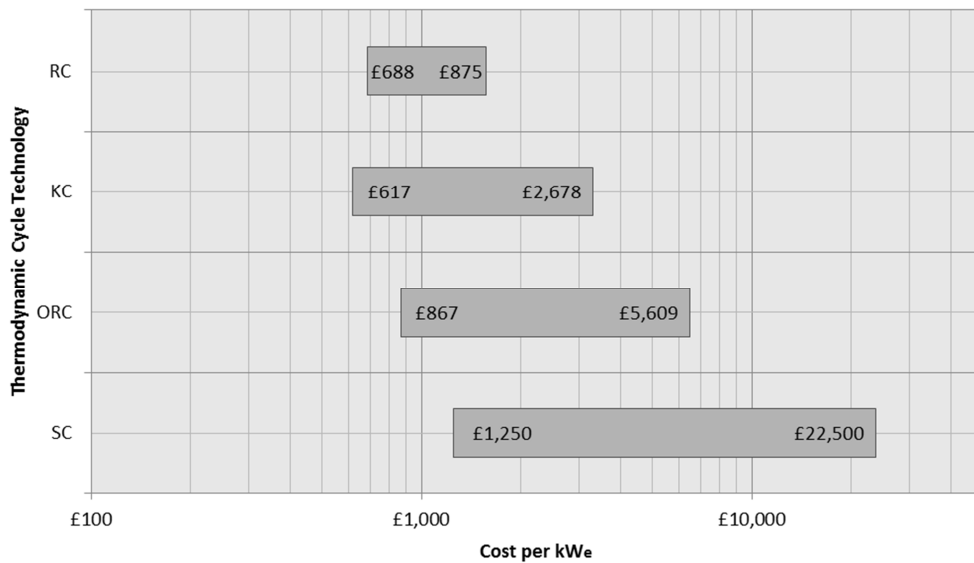
Figure 30: Range of costs per kW e generated for each thermodynamic cycle shown in a logarithm scale found from the available literature.
