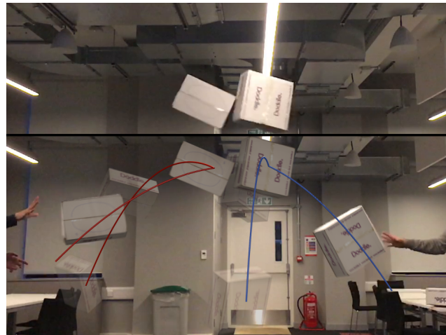
Figure 7: Reconstruction of colliding cuboid shapes from sparsely annotated poses. Top half shows the video at collision time, while the bottom half shows our reconstructed trajectories and selected frames.
