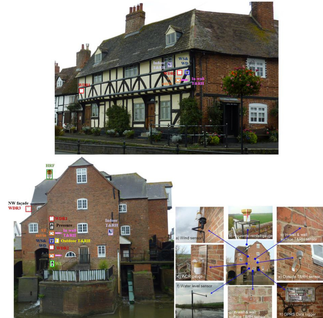
Fig. 2. Schematic position of the sensors installed on the north-western façade of 1-Mill Bank and the south-western and north-western façades of Abbey Mill (WDR: Wind-Drive Rain Gauge, HRF: Horizontal Rain Fall Gauge, WS&WD: Wind Speed and Wind Direction Gauge, ST: Surface Temperature Sensor, WL: Water Level Sensor).
