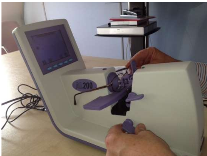
Figure 23 Focimeter with glasses in place to measure the right lens
