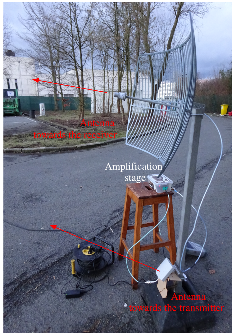
Figure D.1: Photograph of the developed active bistatic transponder.
