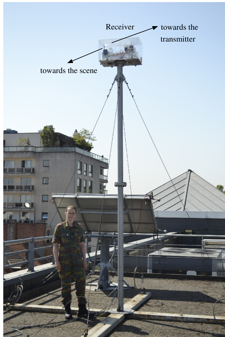
Figure C.2: Photograph of the receiver at the Royal Military Academy located on a mast having a height of 4 m.
