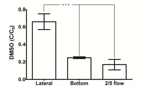
Lateral flow wash alone shows a limited DMSO reduction. The filter device was operated for 10 minutes in the wash mode with a 2 mL/min bottom flow rate without cross flow (20 mL, n=3), with a 5 mL/min lateral flow rate without bottom flow (Lateral 5 mL/min, n=3) and with a 2 mL/min bottom flow rate and a 5 mL/min cross flow rate (2/5 flow, n=6). \*\*\*, p<0.001 (Tukey's multicomparison test).  $254x190mm (96 \times 96 \text{ DPI})$
