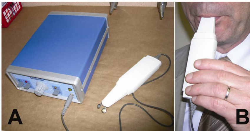
Figure 8-1 First generation electrostimulating device, consisting of a console (A) and a hand-held probe (B)
