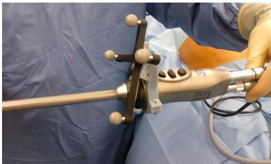
Fig. 1 3D printed tracking collar used in surgery prior to covering in a sterile sheath
