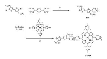
Scheme 2: Synthesis of the TTP and Pt-TTP polymers, (i)  $Pd(PPh_3)_4$ , base, toluene, Ar,  $115^{\circ}C$
