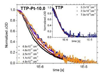
**Figure 7**: Decay dynamics of the triplet excitons at different initial triplet densities for TTP-Pt-10. The inset shows the corrresponding kinetics of the neat TTP polymer. The densities were calculated on the basis of the extinction coefficient of the TTP triplet exciton and the film thickness.
