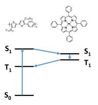
**Figure 1**: Triplet sensitization of a conjugated polymer using a heavy metal complex
