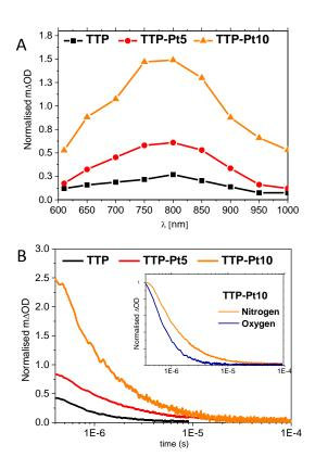
**Figure 3**: Transient absorption spectra of TTP, TTP-Pt-5 and TTP-Pt-10 measured at 800 ns after photoexcitation (420nm) (A) and the corresponding decay dynamics measured at 800 nm (B). The insert in (B) shows the effect of moving from a nitrogen atmosphere (used for all experiments unless otherwise stated) to oxygen for TTP-Pt-10. Analogous acceleration of decay dynamics in the presence of oxygen were observed for all three polymers.
