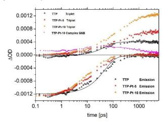
**Figure 5**: Dynamics of spectral features observed from transient absorption spectra such as that shown in figure 4, comprising the 525 nm stimulated emission assigned to TTP singlet excitons (triangles), the photoinduced absorption assigned to TTP triplet excitons (circles) and 510 nm GSB signal assigned to Pt-porphyrin triplet states (dotted line). Lines represent least square fits of these population dynamics using monoexponential functions.
