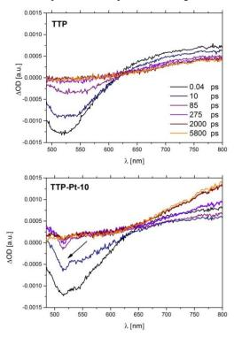
**Figure 4**: TAS spectra of TTP and TTP-Pt-10 films at delay times of 0.04 - 5800 ps after photoexcitation of the TTP ( $\lambda_{exc}$ : 420nm).
