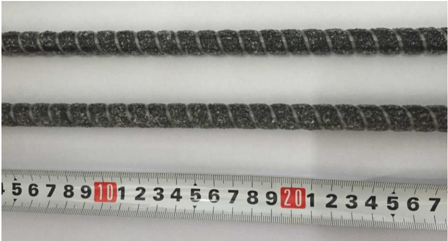
Fig. 2 Basalt FRP bar used for inorganic polymer concrete beams
