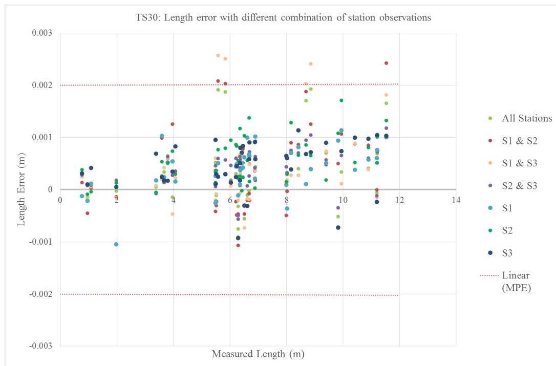
Figure 4.9: Length error of network from different stations with the TS30
