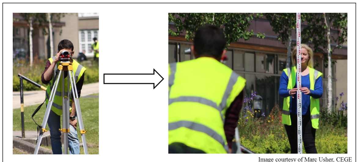
Figure 3.1: Example of automatic levelling: automatic level (left) to read levelling staff (right) at millimetre level
