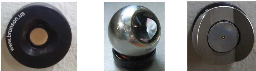
Figure 4.2 a) 1.5" magnetic nest (left); b) 1.5" SMR target (centre); c) 1.5" target adapter (right)
