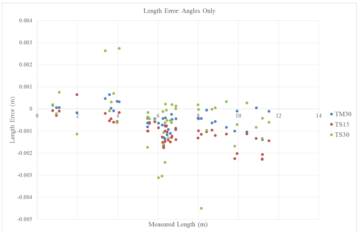
Figure 4.11: Length errors for angles only measurements from total stations
