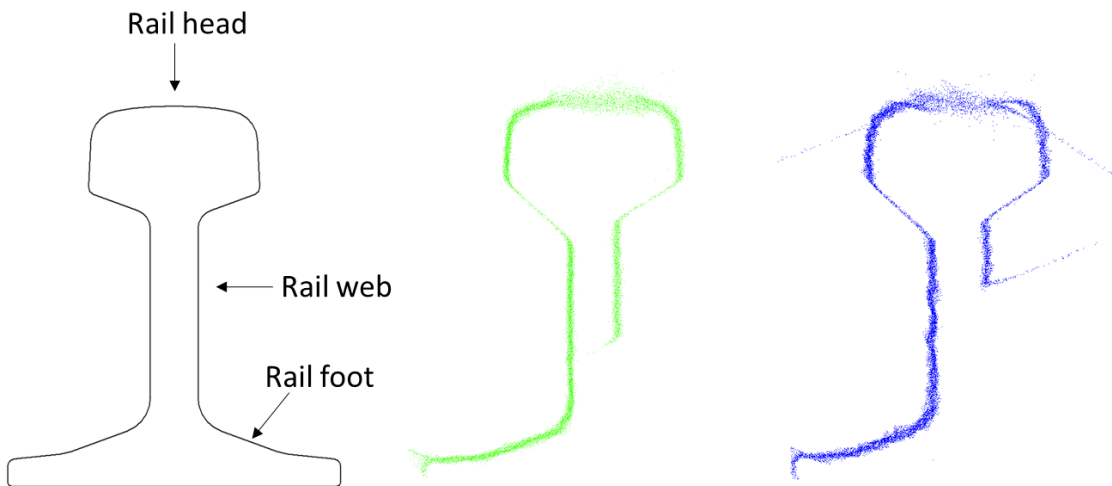
Figure 5.14: Cross-section of rail from the design model, HDS7000 (green) and P20 (blue) laser scanner
