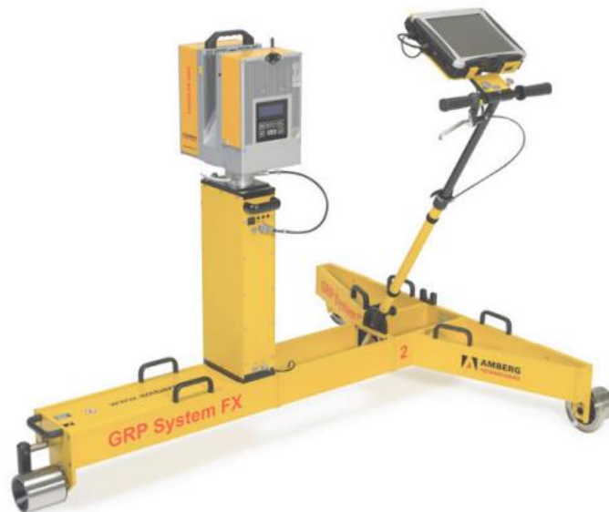
Figure 3.16: Configuration of Amberg Clearance GRP 5000 - image taken from Amberg (2015)
