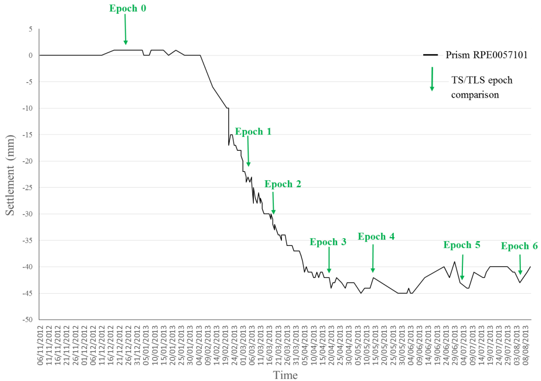
Figure 6.7: Graphical monitoring results from prism target RPE0057101- data taken from Sol Data Geoscope's monitoring database
