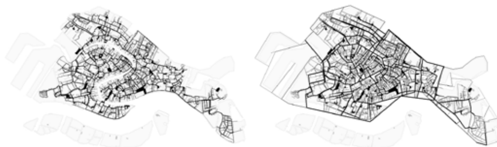
Figure 1. Left: Choice (3000 radius) network of street system. Right: Street-canal system. The two networks intersect in Venice’s squares.
