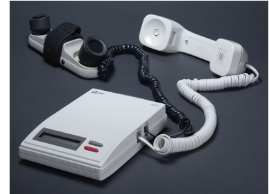
Figure 3: The AT&T TSD-3600E: one voice encryption product based around the Clipper chip. (Photo: Matt Blaze)
