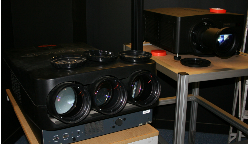
Figure 5.4: Projectors used in the Cave system. An old CRT projector on the left part of the picture and a new DLP one in the right side.
