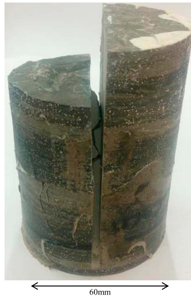
Figure 9. An Arrestor-orientation short-rod sample which has succumbed to transverse tensile failure. The fracture has progressed along the chevron plane until it reaches a point where less energy is required to propagate the fracture perpendicular to the axis of the cylinder. This occurred commonly during Arrestor-orientation experiments. This is a manifestation of the same effect as is seen to divert the Arrestor orientation cracks during Brazilian Disk tests in Figure 6.
