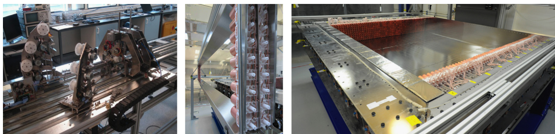
Fig. 3. The wiring robot (left), a cassette being inspected before installation (center), and the first quarter of the Demonstrator Module after completion (right).
