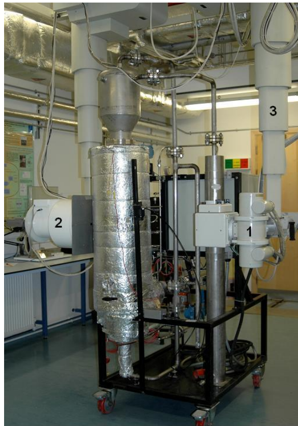
Figure 3.6: Experimental set-up showing the x-ray machine employed to visualize the bed. 1: x-ray generator 2: x-ray tube 3: image intensifier.
