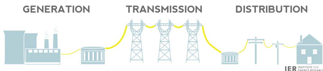
Figure 3-1: Diagram of a centralized electricity system (reproduced from Institute for Energy Research 10 ).
