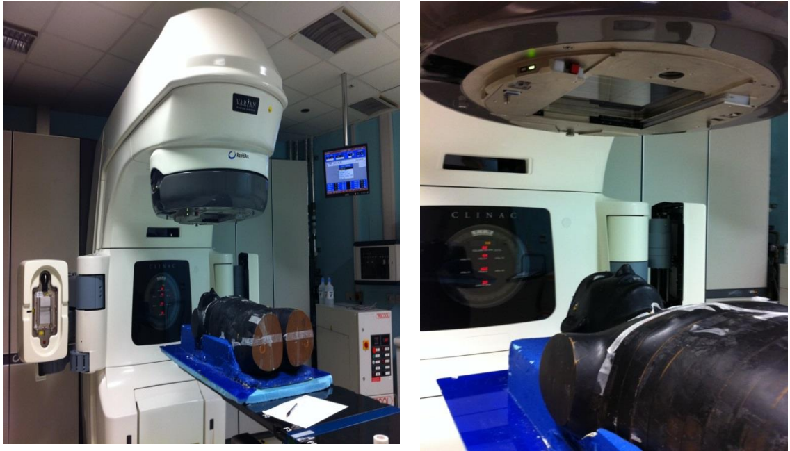
Fig. 3.9: A Rando-phantom used to demonstrate dose to areas outside target volume with typical SF-IMRT, RA and CRT plans.
