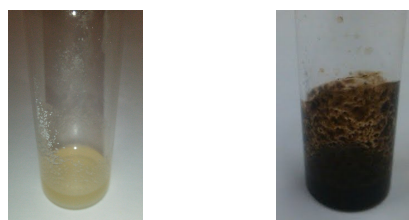
Figure 1: Demonstration of reactivity of KOtBu when mixed with (a) commercial 1,10-phenanthroline and (b) Purified 1,10-phenanthroline
